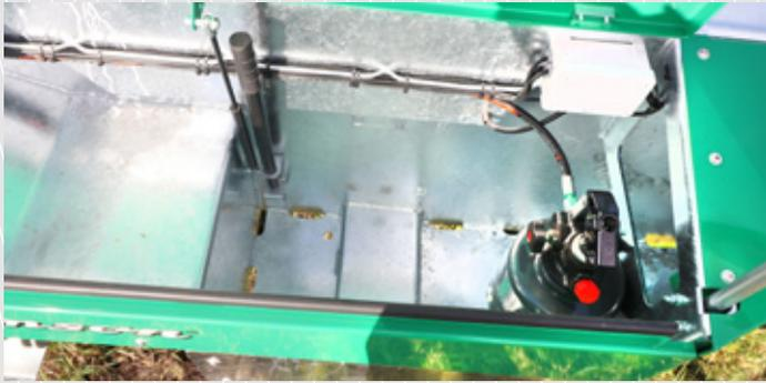
The hand pump is well protected in the storage compartment.
