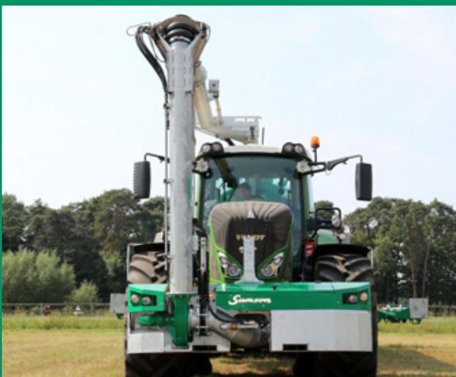
*Side-mounted filling arm ensures optimal visibility from the cab.*
