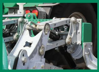
The parallelogram hitch ensures precise depth control for each row. This means the slurry is always placed at the preset height.
