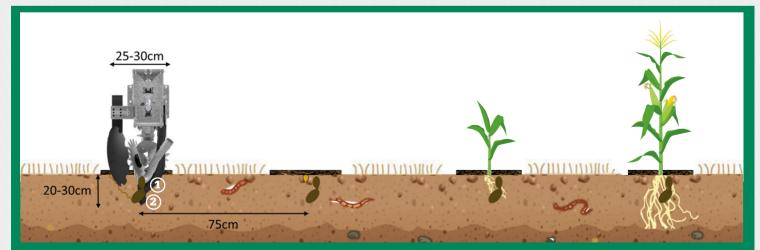
SAMSON Strip-Till workflow is functional and extremely precise. The slurry is placed in two lines: (1) approx. 30 % in the upper and (2) approx. 70 % in the lower slurry line.
