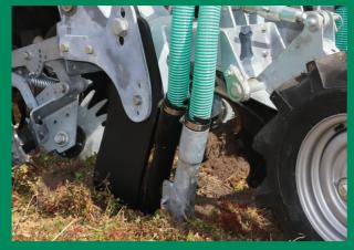
Specially developed nozzles with integrated slurry hoses place the slurry precisely behind the tooth. The nozzles can be adjusted easily and the placing of slurry lines can be adapted.
