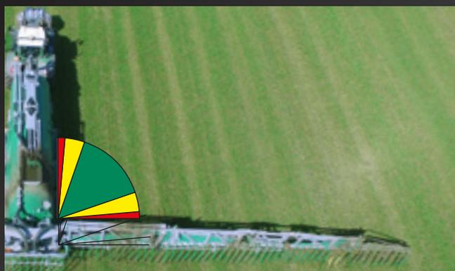
Angle sensors control the speed of the inner wings during folding. Green: Max. speed, Yellow: Reduced speed and Red: Boom stops.
