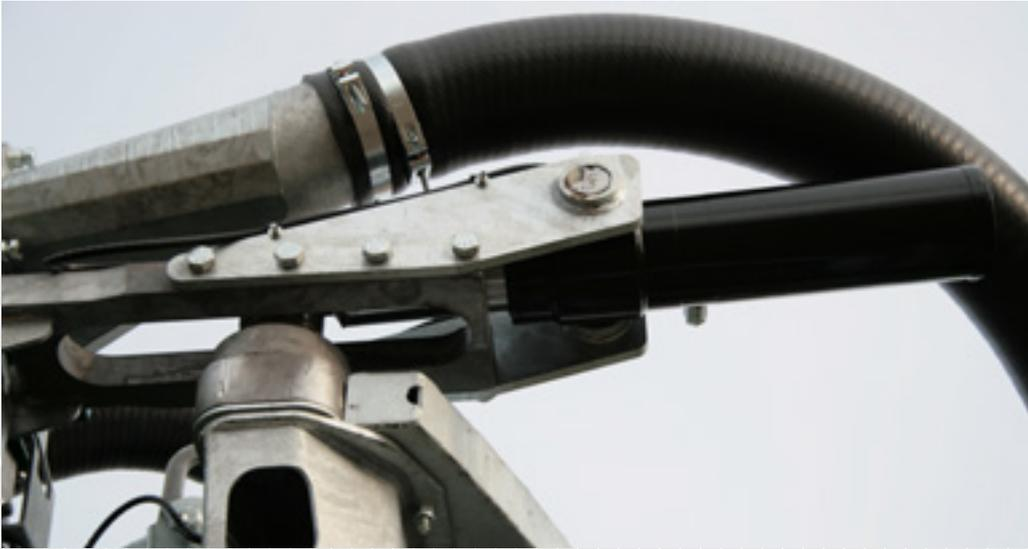
*The two large side wings are hinged at the bottom and are controlled by a large hydraulic cylinder at the top.*
