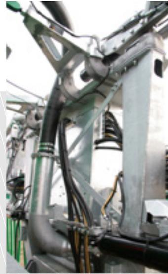
*The boom has a simple central frame with no moving parts.*
