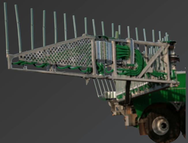
*The new drip stop rotates the hoses so they point upwards.*
