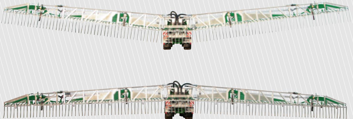
*The side wings of the SHB4-36m boom can be adjusted individually both above and below level in relation to the central frame.*
