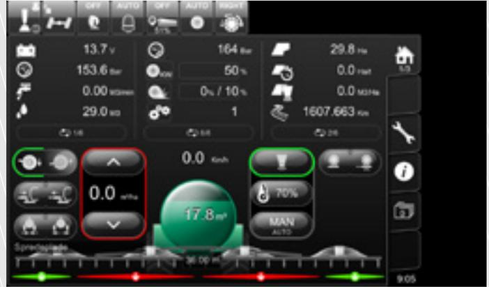
It is very easy to operate the new boom via the SlurryMaster 8000 control system. You can always see which distributors are in use.
