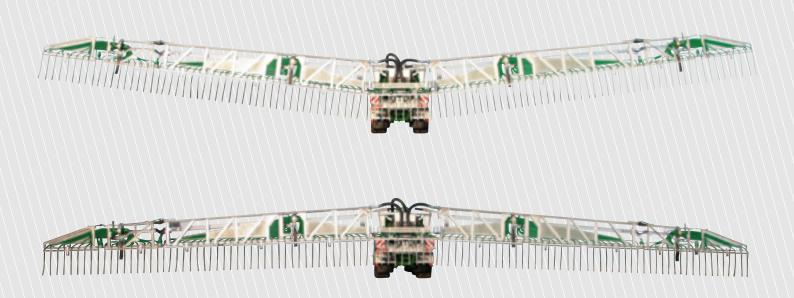
The side wings of the SHB4-36m boom can be adjusted individually both above and below level in relation to the central frame.
