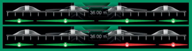
Sections can be closed off for each distributer. When sections are closed off, the amount of slurry is adjusted so dosing remains constant.
