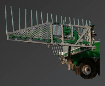
The new drip stop rotates the hoses so they point upwards.
