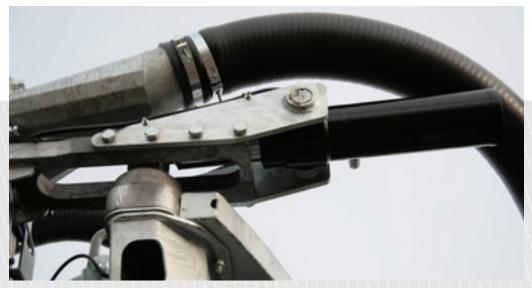
The two large side wings are hinged at the bottom and are controlled by a large hydraulic cylinder at the top.
