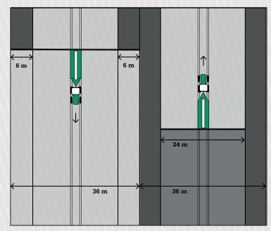
First pass: Slurry is applied on the outer 6 metres.
