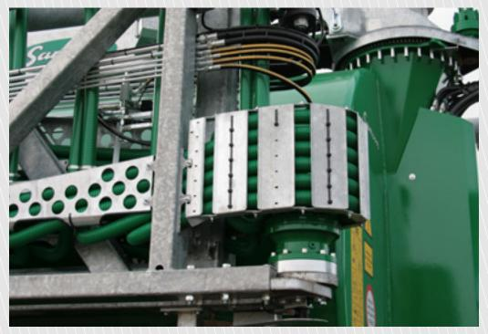
The side wings are folded in two layers using a planetary gear driven by an oil motor.
