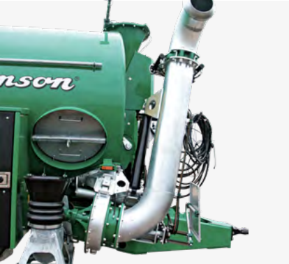
SAP 1* Single link side-mounted filling arm with integrated pump. Simple and fast filling of the slurry tanker from a low funnel.
