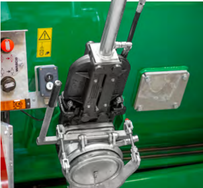
Filling coupling with hydraulic slide valve* Integrated filling coupling provides fast access to filling directly via the SAMSON ejector*. Fitted with quick coupler for the hoses and hydraulic slide valve* with external control.
