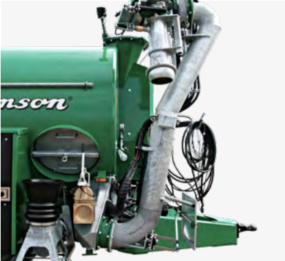
SAP 2* Double link side-mounted filling arm with integrated pump. Universal filling arm with the option of filling from a low or high filling funnel with a coupling and from difficult to access slurry stores.
